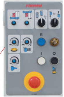
Traditional OP1 operating panel
